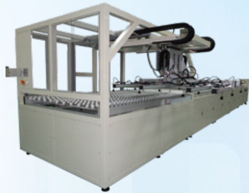
移載送板機構 (TRANSFER LOADER)
